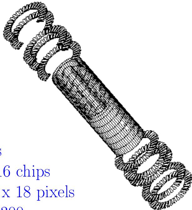
Fluence of  $10^{15}\text{neq}/\text{cm}^2$  for the innermost layer after 5 years
