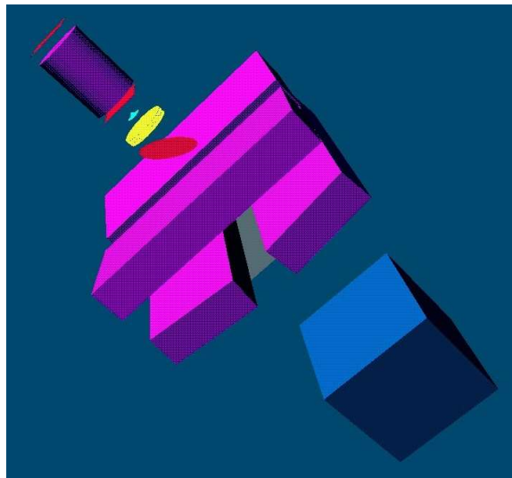
Figure 5: The geometry of a treatment head for Intensity Modulated RadioTherapy (IMRT).
