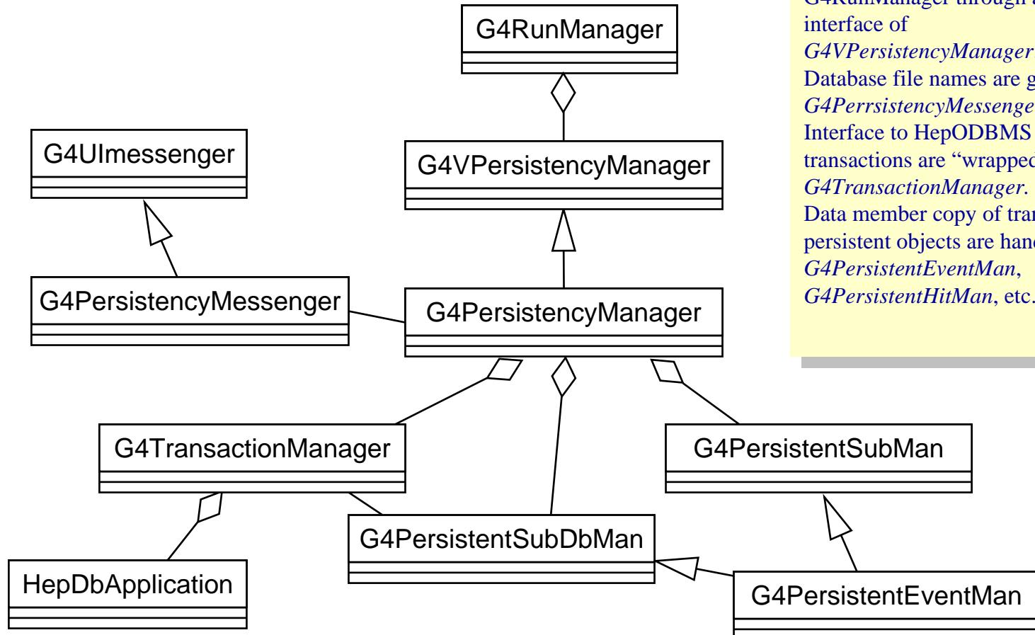
Transient G4 objects are “stored” by **G4RunManager** through abstract interface of **G4VPersistenceManager**. Database file names are given via **G4PersistenceMessenger**. Interface to HepODBMS transactions are “wrapped” at **G4TransactionManager**. Data member copy of transient and persistent objects are handled by **G4PersistentEventMan**, **G4PersistentHitMan**, etc.
