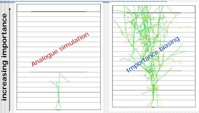
10 MeV neutron in thick concrete cylinder Biasing and scoring - Geant4 Course
