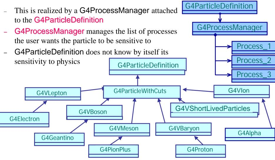
G4ParticleDefinition is the base class for defining concrete particles
