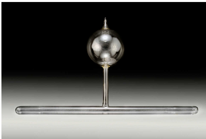
Figure 4.2: Shown is one of the glass polarized ^3\text{He} target cells used during GEN-I (E02-013). These were the first polarized ^3\text{He} target cells used in electron scattering to incorporate alkali-hybrid technology.
