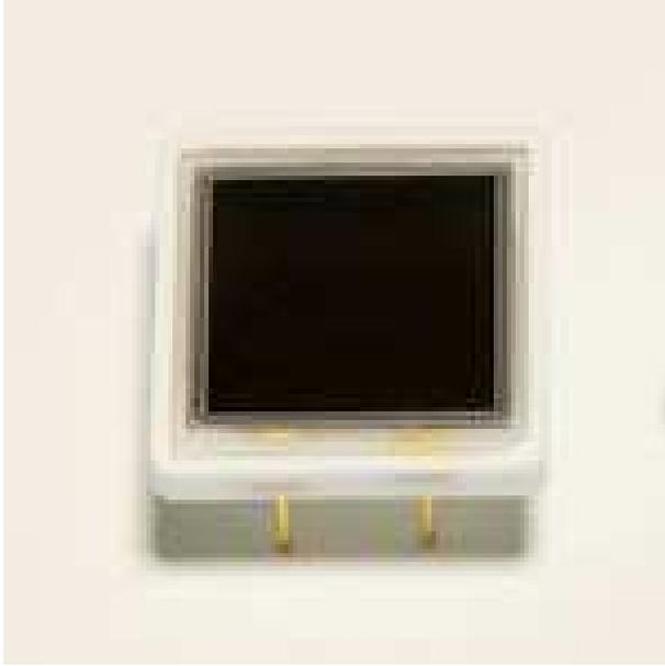
Figure 23: The Hamamatsu Photonics s8664-1010 Large Area APD.
