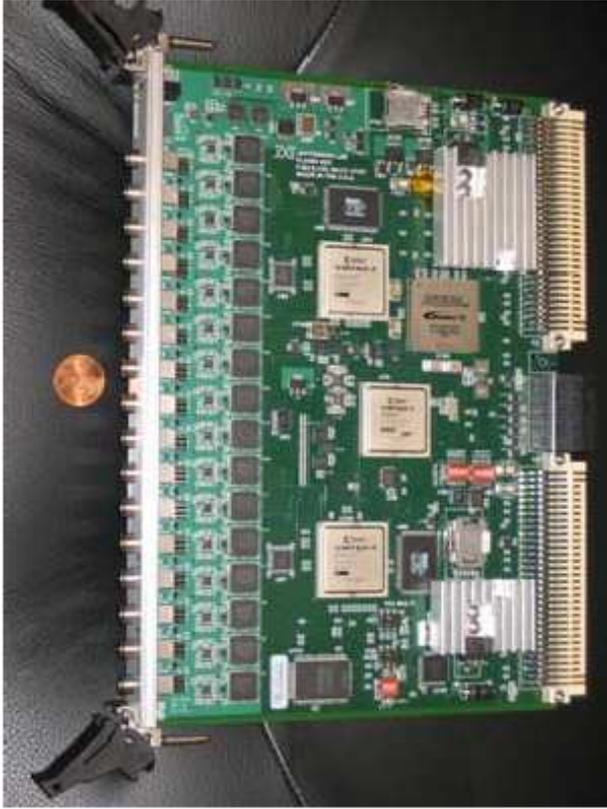
Figure 49: The JLab fADC.
