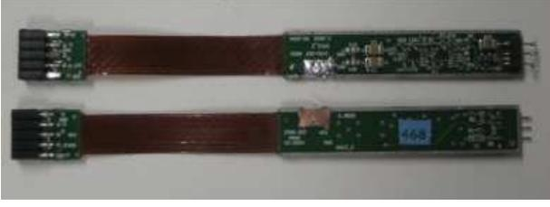
Figure 39: Front and rear view of an amplifier board.
