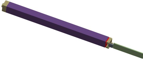
Figure 50: Single crystal assembly: from the front to the back, the PEEK holding nose, the wrapped crystal, the LAAPD in the PEEK housing, the FT-Orsay preamplifiers grounded with a Cu plate.
