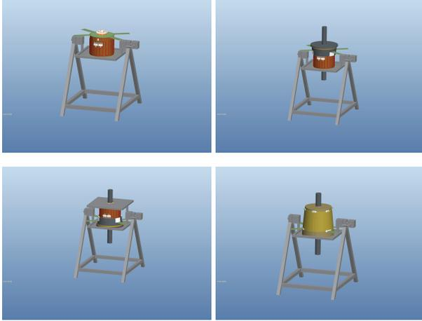
Figure 125: FT mounting procedure, step 2. From top-left: the motherboard on the back side (1), the back tungstane hat (2). Flipping again: the front part is now up-ward looking, inserting the inner tungstane pipe (3), completing with the external thermal insulator (4).
