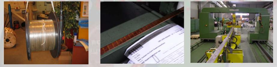
Two lengths are available of the developed low loss conductor: 717 m (Enough for the coil) + 120 m used for winding tests . Ic@5T,4.2K= 16740 A (spec.18540 A)  $\rightarrow$  0.8 K margin (1 K).
