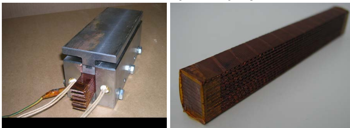
FIG.139: Stacked conductor ready to be cured, on the left, and a cured sample, on the right.
