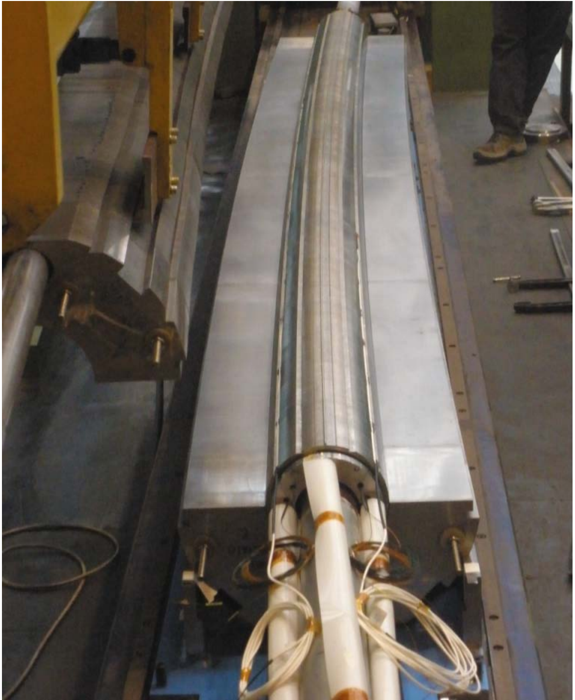
FIG.113: Lower half yoke hosting the collared coil. Both halves of the yoke are composed of four large blocks in silicon steel and two small blocks in stainless steel at the magnet ends.
