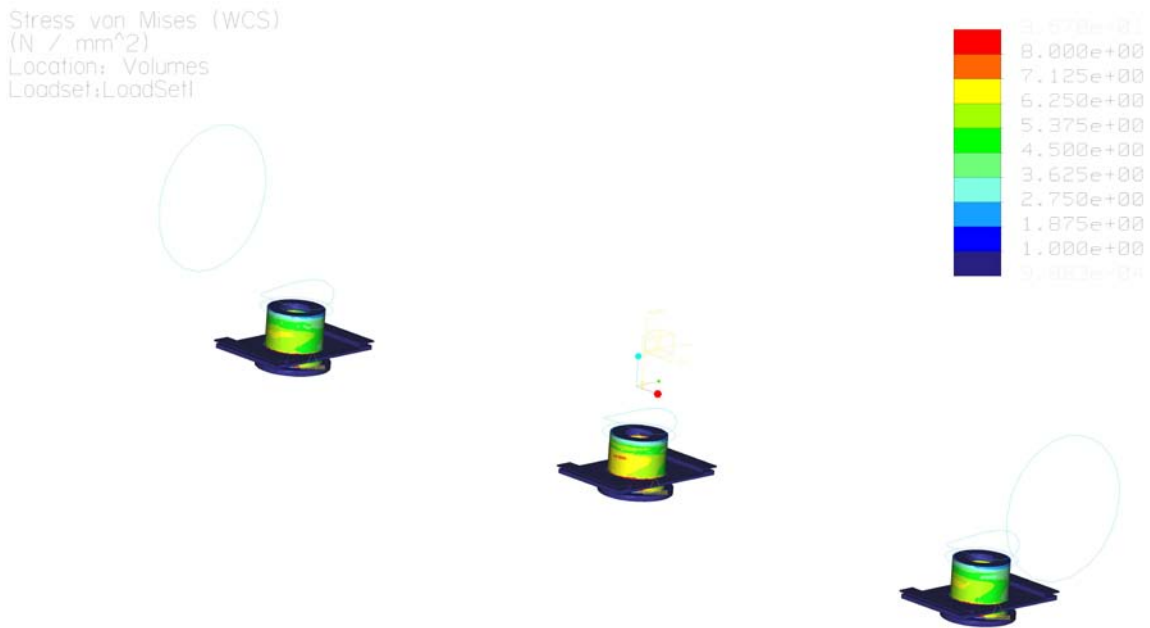
FIG.92: Stress analysis among POSTs placed “in line” at maximum distance from the centre.
