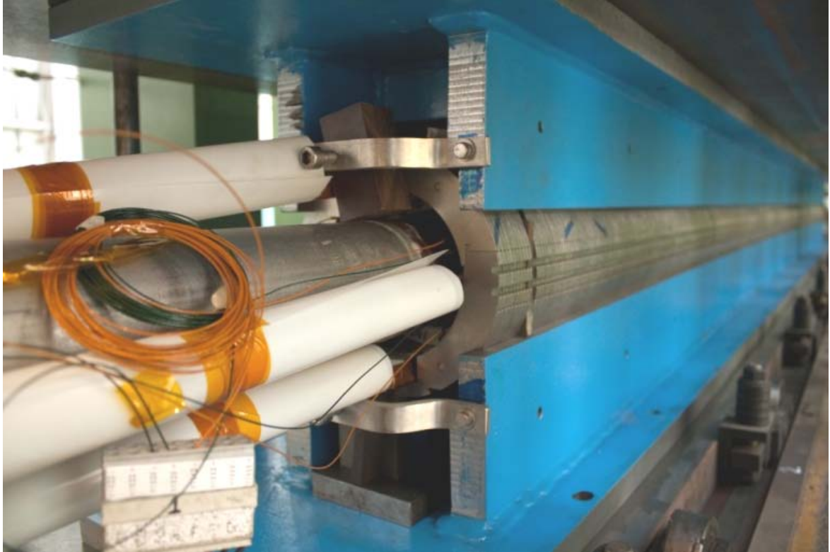
FIG.112: The coil inside the press during the collaring operation. The photo captures the moment when the cavities housing the keys on the collars are aligned.
