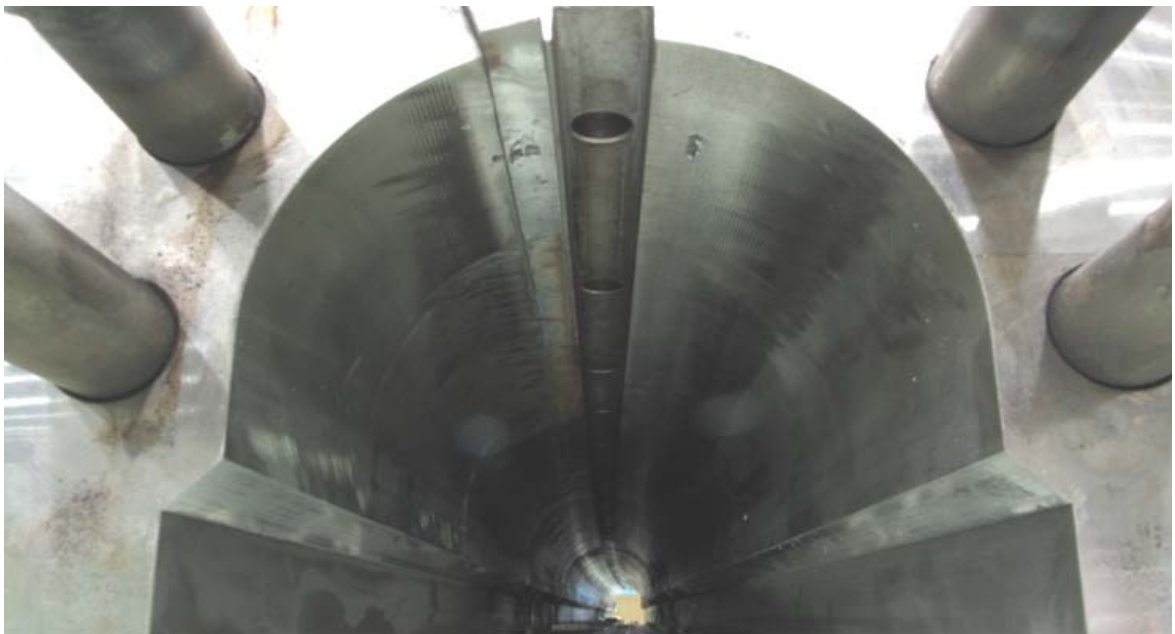
FIG.110: The mold for coil curing under pressure. The geometrical curvature is clearly shown.
