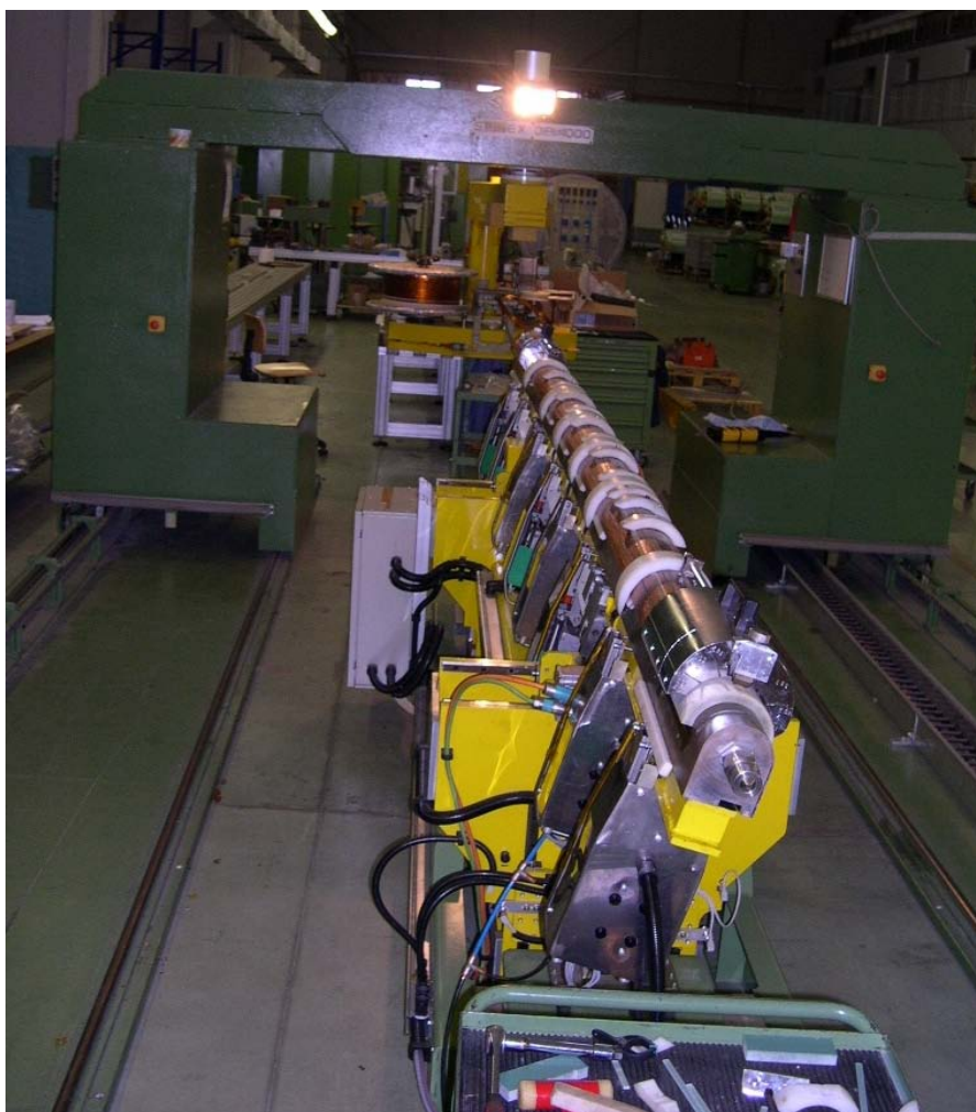
FIG.103: Winding operation with a dummy conductor. The geometrical curvature is clearly appreciable.
