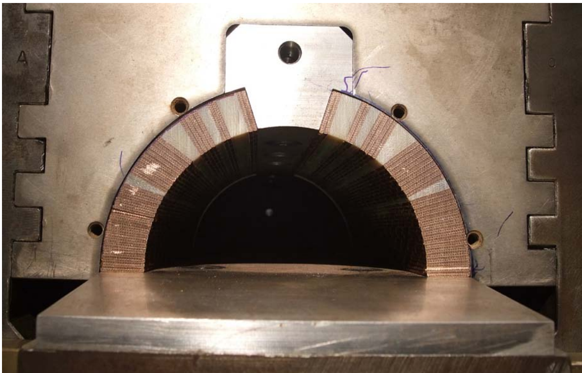
FIG.142: Arc piled sample for stress-strain measurements.
