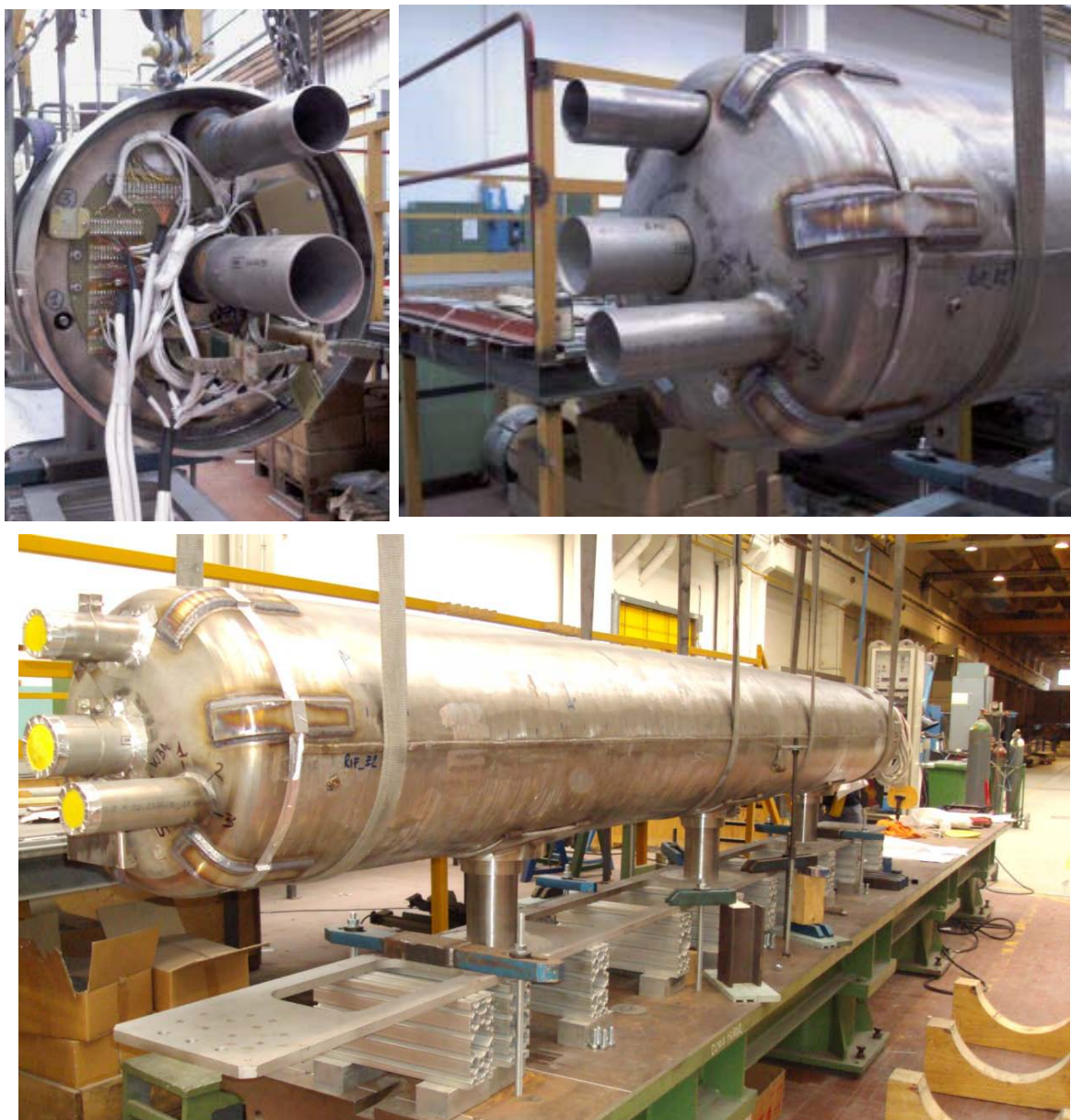
FIG.115: .The cold mass as finished and stored in ASG-Superconductors (lower figure) . In a first time the end caps flanges (the doomed ones) were not welded in definitive way but only with a temporary welding. The final welding was done after the test at LASA. In this way we had th possibility to correct the axial pre-stress if required. In the upper figure on the left the coil end is shown with bus bars and instrumentation wires before the doomed flange was welded
