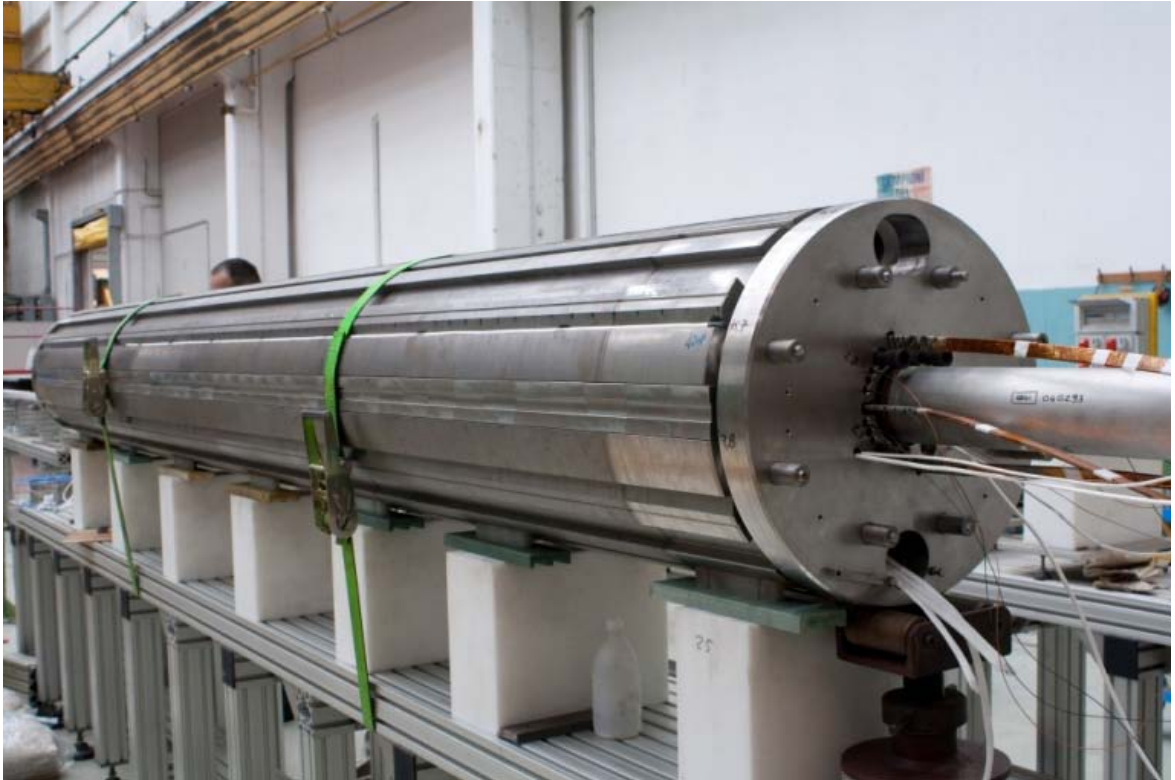
FIG.114: . The magnet as it appears after integration into the iron yoke. At the mid-plane the c-clamps holding the two halves of the yoke can be seen
