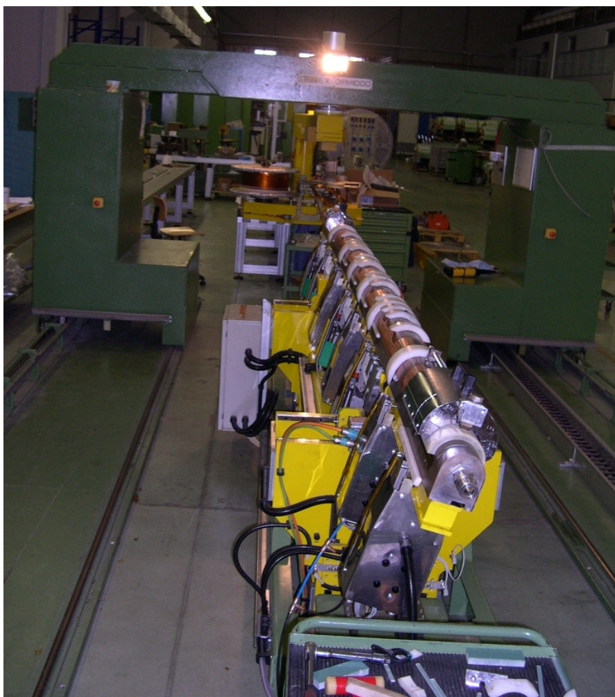
FIG.74: Winding operation with a dummy conductor. The geometrical curvature is clearly appreciable.
