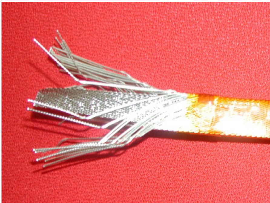
FIG.5: The 36 strand Rutherford cable. In between the strands one can see the thin stainless steel core used for depressing the inter-strand coupling currents.
