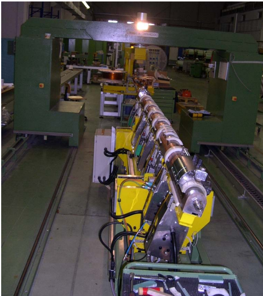
FIG.85: Winding operation with a dummy conductor. The geometrical curvature is clearly appreciable.
