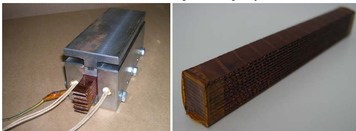
FIG.115: Stacked conductor ready to be cured, on the left, and a cured sample, on the right.
