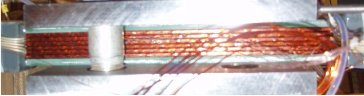
FIG.66: The sample used for thermal heat measurements through the kapton insulation.
