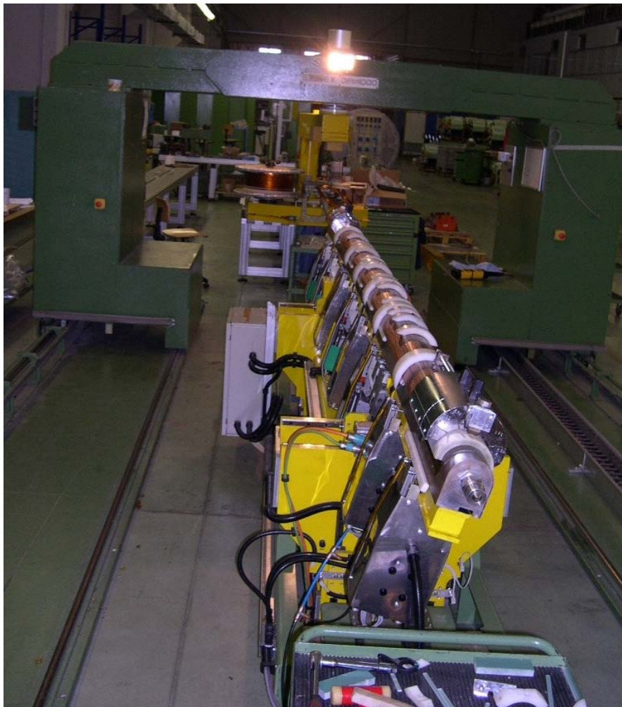
FIG.85: Winding operation with a dummy conductor. The geometrical curvature is clearly appreciable.
