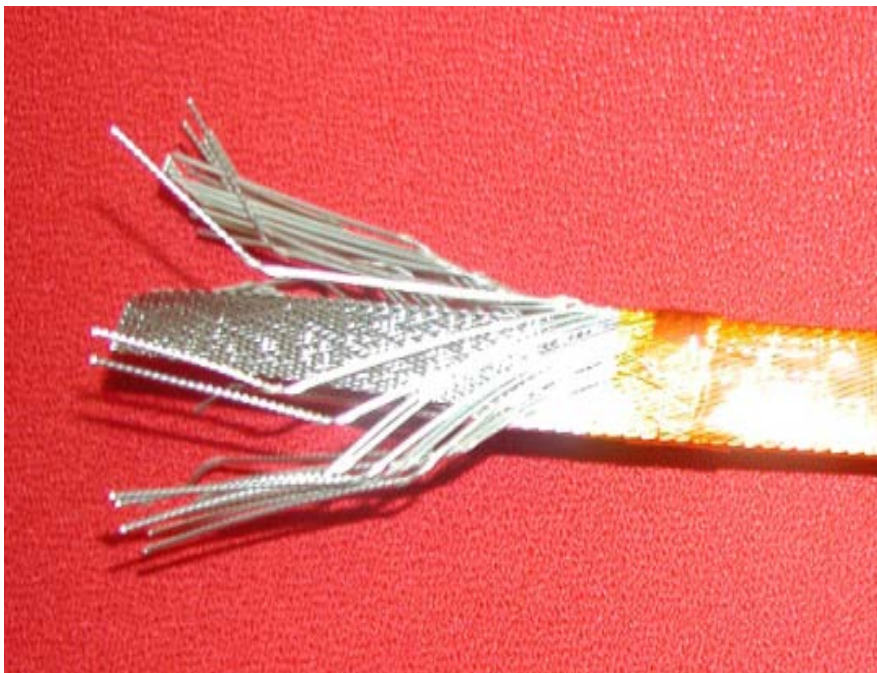
FIG.6: The 36 strand Rutherford cable. In between the strands one can see the thin stainless steel core used for depressing the inter-strand coupling currents.
