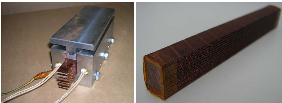
FIG.120: Stacked conductor ready to be cured, on the left, and a cured sample, on the right.
