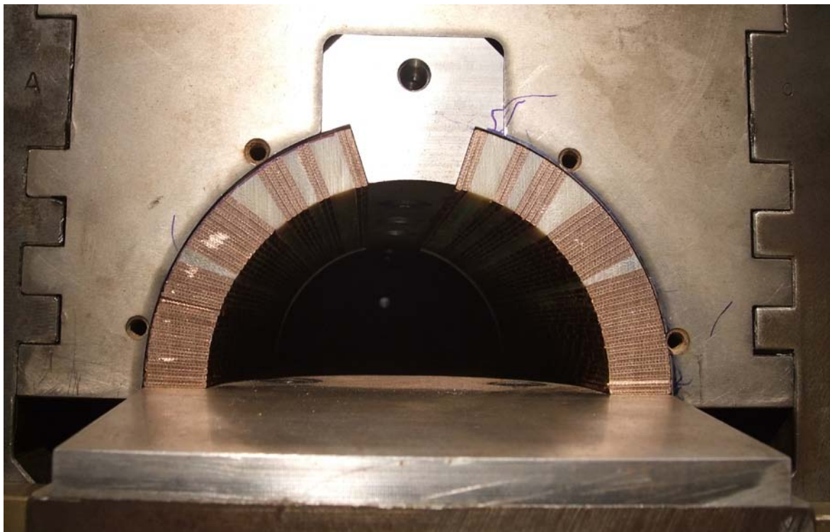
FIG.123: Arc piled sample for stress-strain measurements.
