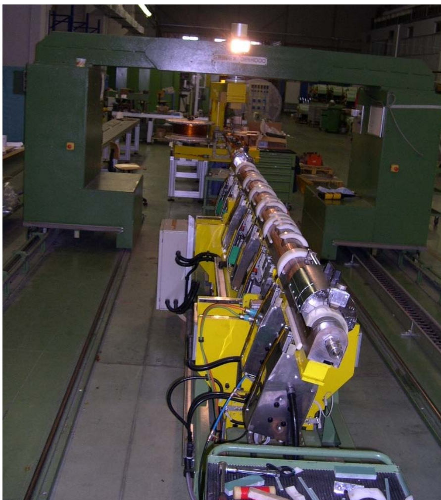
FIG.90: Winding operation with a dummy conductor. The geometrical curvature is clearly appreciable.
