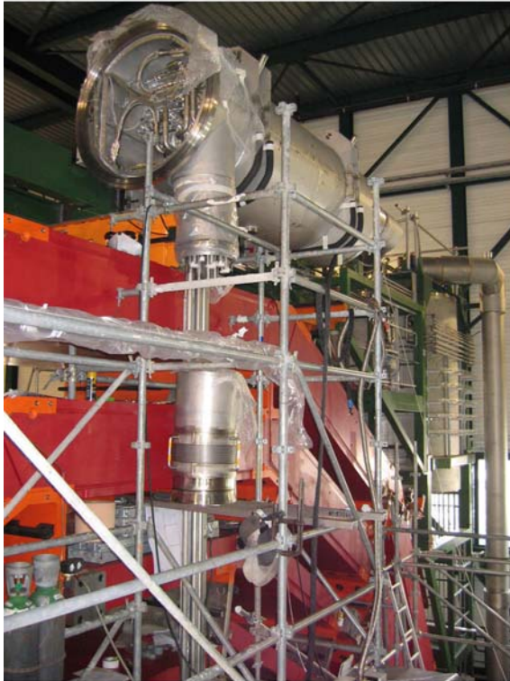
The cryogenic chimney links the cold mass to the phase separator cryostat by SDMS (F)
