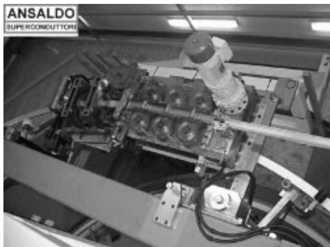
Fig. 5. The constructed two-step pre-bending unit under test.
