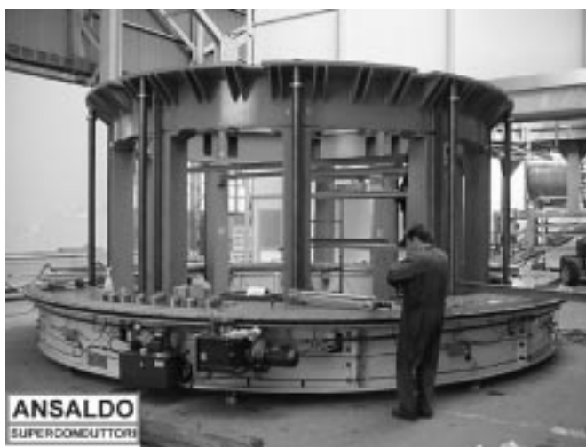
Fig. 8. Winding table with fixed and rotating parts and lifting system.
