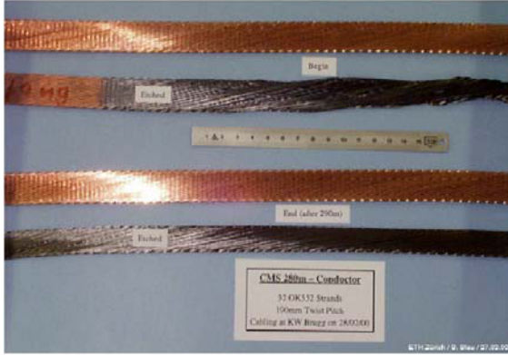
Figure 2. Several strands are assembled through a cabling process to give the flat Rutherford cable (Case of CMS conductor made from 36 strands)
