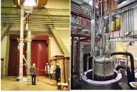
Fig. 1. Magnet and movement tool just rotated in the vertical position (left) and insertion of the magnet in the vertical cryostat (right).
