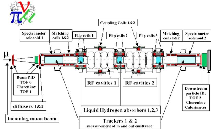
Fig. 1. A cross-section representation of MICE. The tracker magnet is a combination of two matching coils plus a three-coil spectrometer solenoid that is around the tracker. Not shown are the iron shields at the tracker magnet ends. The AFC module is described as flip coils, even though the polarity of the coils in the AFC module may be either in the flip or non-flip mode. The coupling coils are around the RF cavities in the RFCC module.
