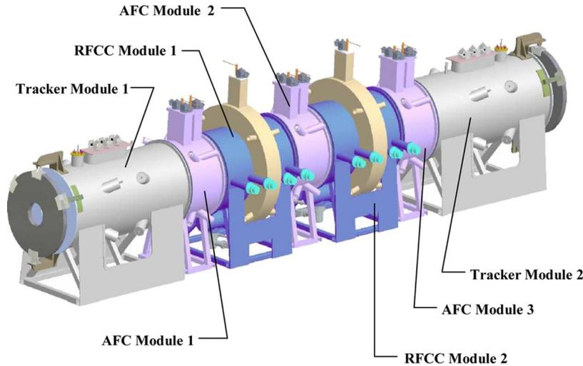
Fig. 2. A three-dimensional schematic representation of the MICE channel with three AFC modules and two RFCC modules.
