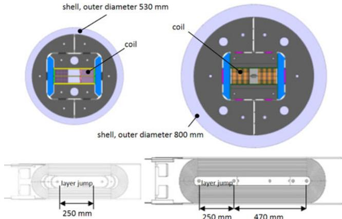
Fig. 1. Comparison between RMC (left) and ERMC (right) layouts
