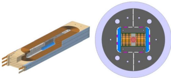
Fig. 2. RMM: 3D view of the coils and 2D cross section of the structure
