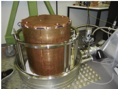
**Fig. 3.** The copper heat exchanger and its support.
