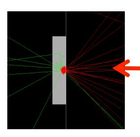
Physical expectation: a fraction of electrons is backscattered (consistent with experiment)
