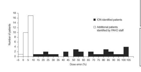
The software permitted incorrect forms of data entry, which in turn led to miscalculation of treatment time
