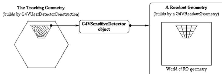
**Figure 4.8. Association of tracking and readout geometry.**
