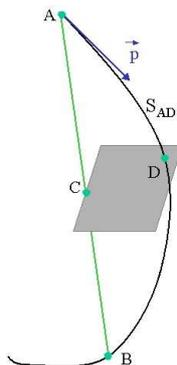
**Figure 4.7.** The distance between the calculated chord intersection point C and a computed curve point D is used to determine whether C is an accurate representation of the intersection of the curved path ADB with a volume boundary. Here CD is likely too large, and a new intersection on the chord AD will be calculated.
