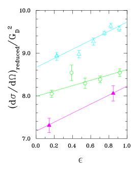
Figure 3: Demonstration of the Rosenbluth separation method based on the data from [And94]. The  $Q^2$ values shown are 2.5 (open triangle), 5.0 (circle) and 7.0 (filled triangles)  $GeV^2$ .
