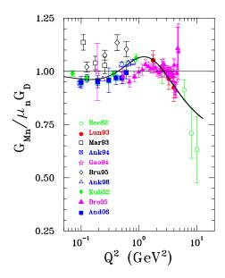
Figure 21: The complete data base for  $G_{Mn}$ , from cross section and polarization measurements. Shown as a solid curve is the polynomial fit by Kelly [Kel04]; note that the recent data of [Bro05] are not included in this fit.
