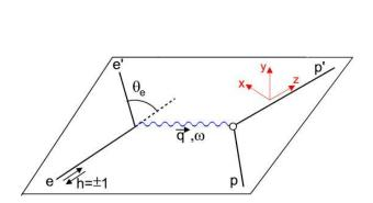
Figure 14: Kinematical variables for polarization transfer from a longitudinally polarized electron to a proton with exchange of a virtual photon.
