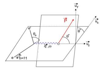
Figure 15: Polarized electron scattering from a polarized target.
