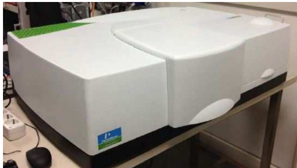
Figure 14: The Lambda 650 S PerkinElmer spectrophotometer used for the aerogel characterization.
