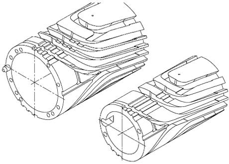
Fig. 56. Drawing of the coil tube ends. End Lorentz forces are contained in the slots.
