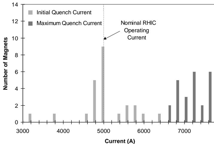
Fig. 42. Quench performance of 24 large aperture (100 mm) dipoles, tested at 4.5 K.
