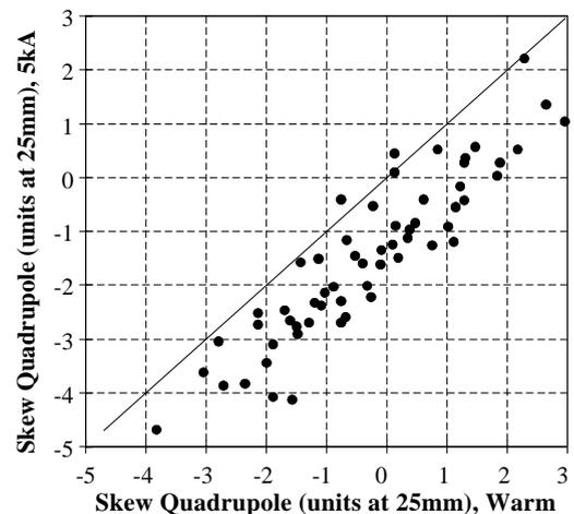
Fig. 5. Measured warm–cold skew quadrupole correlation.
