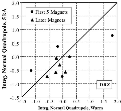
Fig. 43. Warm–cold correlation of the normal quadrupole harmonic ( $b_1$ ) in D0 dipoles.
