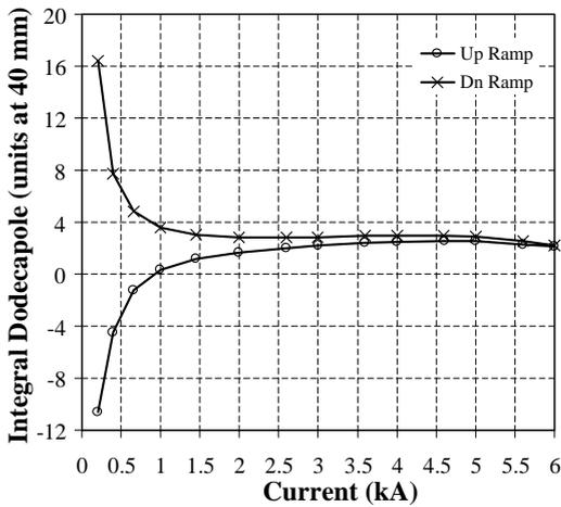
Fig. 33. Integral first allowed harmonic ( $b_5$ ) in Q1 magnet QR1114.
