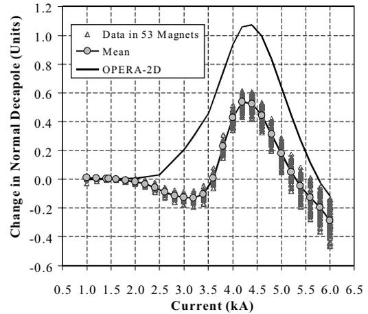
Fig. 11. Current dependence of the normal decapole component.
