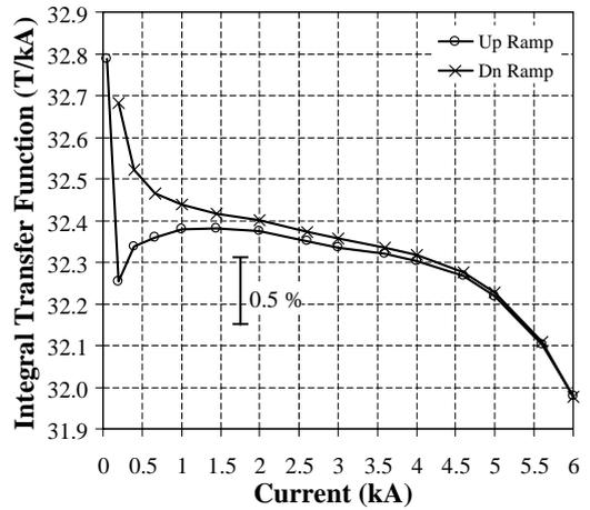
Fig. 34. Integral transfer function in Q2 magnet QRK119 (close to mean at 5 kA).
