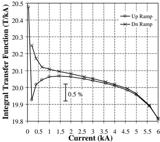
Fig. 36. Integral transfer function in Q3 magnet QRJ116 (close to mean at 5 kA).
