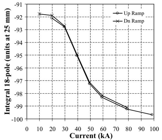
Fig. 21. Integral of the first allowed harmonic ( $b_8$ ) in SRE211.
