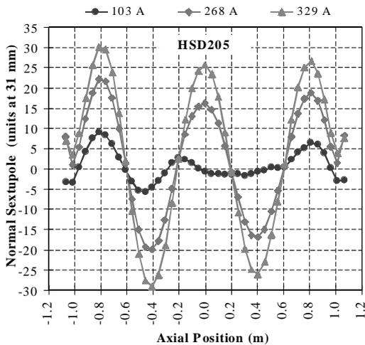
Fig. 64. Normal sextupole harmonic as a function of the axial position in HSD205.
