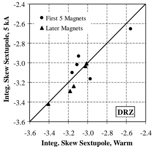
Fig. 46. Warm–cold correlation of the skew sextupole harmonic ( $a_2$ ) in D0 dipoles.
