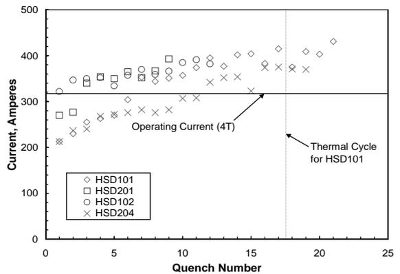
Fig. 58. Quench performance of the four magnets of the first Snake. After some initial training, each reached a current comfortably above the maximum operating point of 4 T. A thermal cycle showed no retraining.
