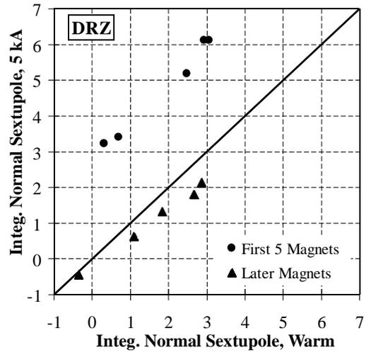
Fig. 45. Warm–cold correlation of the normal sextupole harmonic ( $b_2$ ) in D0 dipoles.
