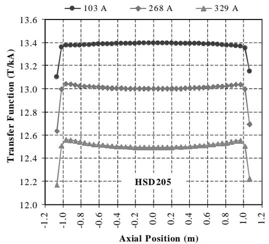
Fig. 62. Axial scan of the transfer function in HSD205.
