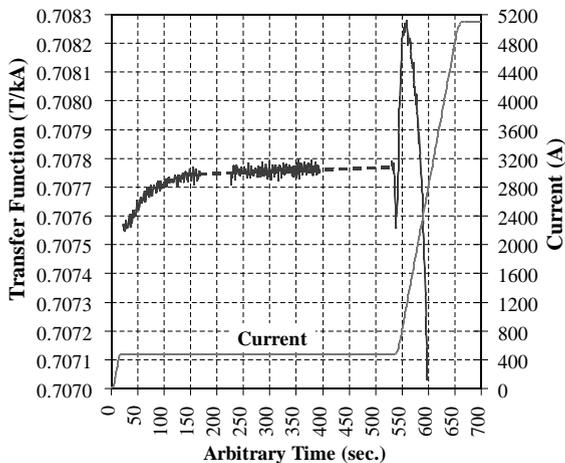
Fig. 13. Time decay and snapback in D96525.
