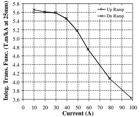
Fig. 20. Integral transfer function in SRE211.
