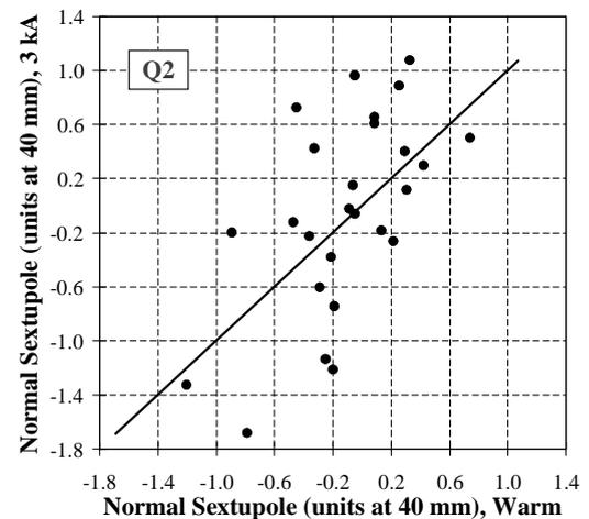
Fig. 39. Warm-cold correlation of  $b_2$  in the Q2 (QRK) magnets at 3 kA.
