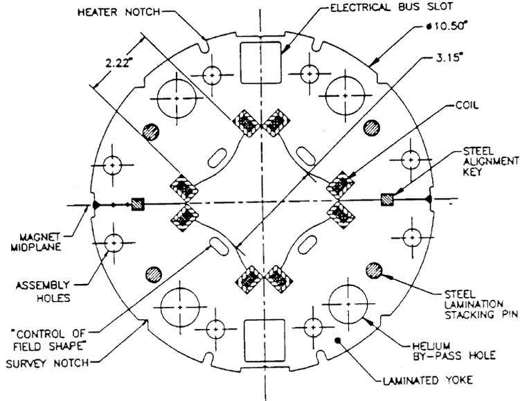
Fig. 22. Cross-section of the trim quadrupole magnet.
