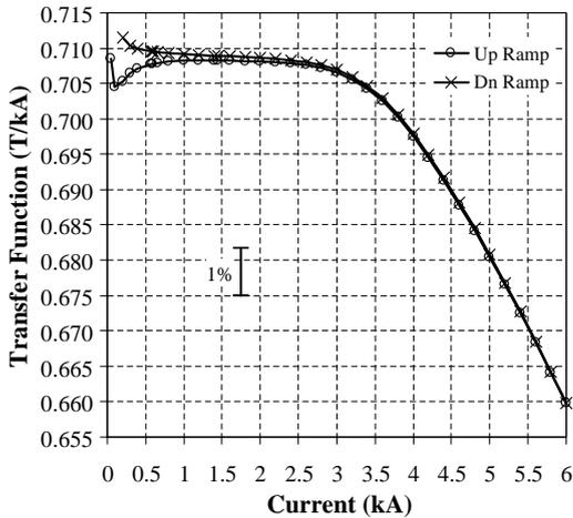
Fig. 12. Transfer function for a typical 80mm dipole in the straight section.
