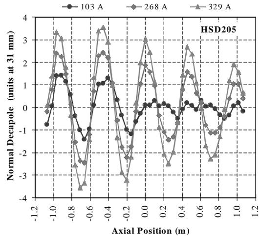
Fig. 65. Normal decapole harmonic as a function of the axial position in HSD205.
