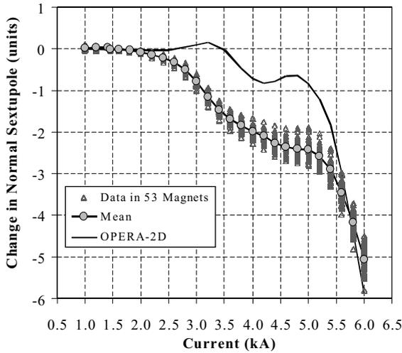
Fig. 10. Current dependence of the normal sextupole component.
