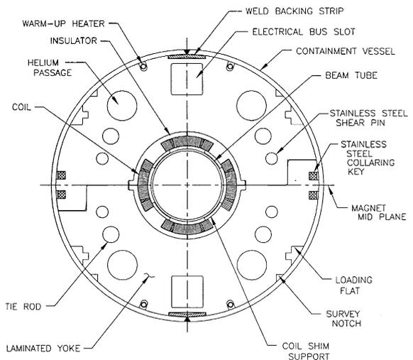
Fig. 14. Cross-section of the arc quadrupole magnet.
