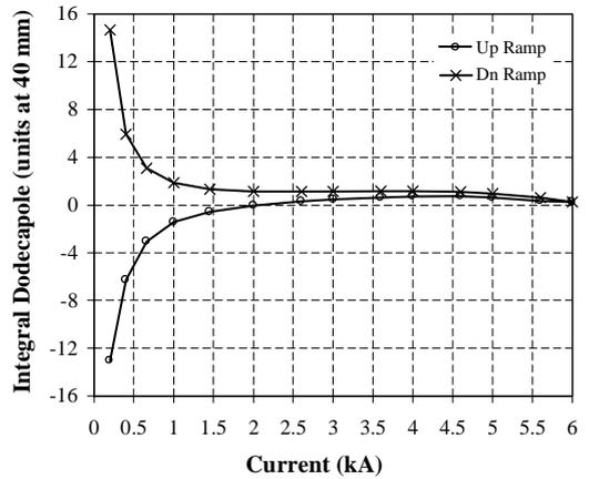
Fig. 35. Integral first allowed harmonic ( $b_5$ ) in Q2 magnet QRK119.
