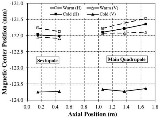
Fig. 29. Correlation between warm and cold centers in a CQS assembly.
