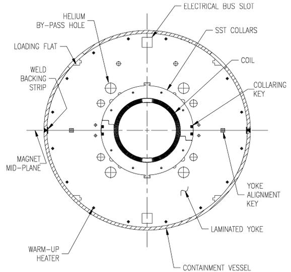
Fig. 48. Cross-section of the 180 mm DX dipole magnet.
