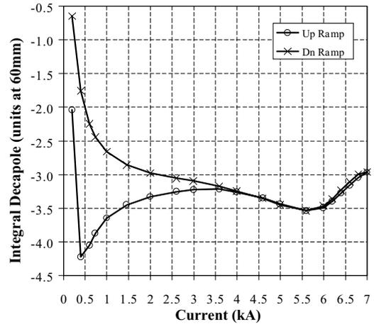
Fig. 52. Integral normal decapole harmonic in DRX110.
