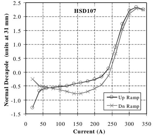
Fig. 61. Normal decapole harmonic at the center of HSD107.
