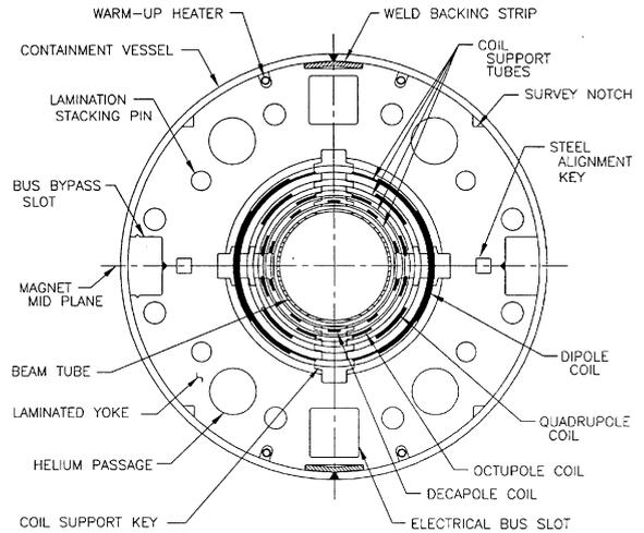
Fig. 25. Cross-section of the 80 mm corrector magnet.
