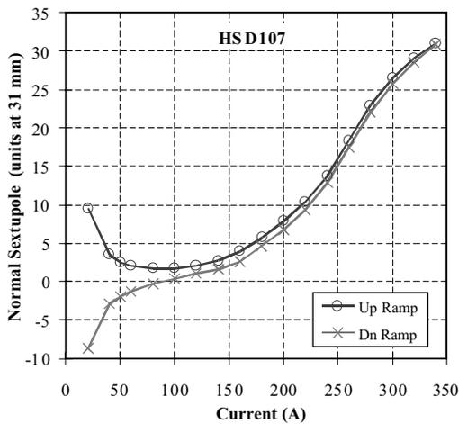
Fig. 60. Normal sextupole harmonic at the center of HSD107.
