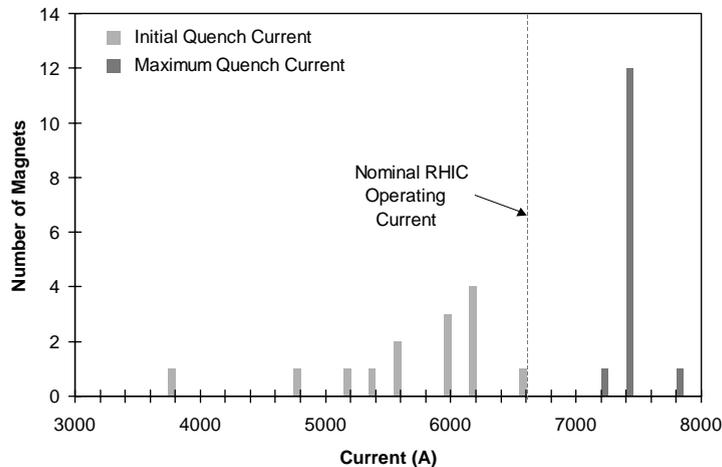
Fig. 49. Quench performance of 14 large aperture (180 mm) dipoles, tested at 4.5 K.
