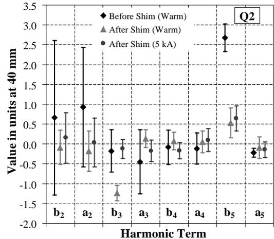
Fig. 38. Harmonics before and after shimming in the Q2 quads (QRK).
