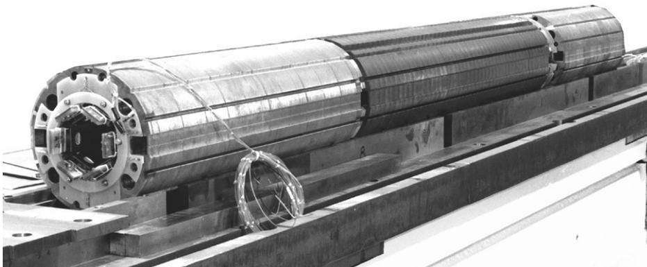
Fig. 27. The magnets of a CQS unit on the assembly bench. In the foreground is a sextupole cold mass, followed by quadrupole and corrector cold masses.
