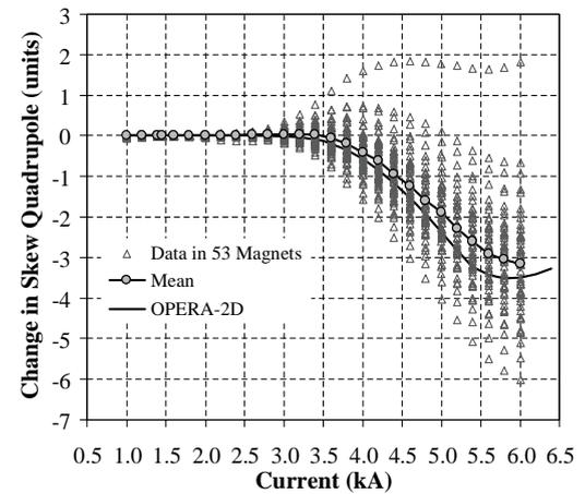
Fig. 9. Current dependence of the skew quadrupole component.
