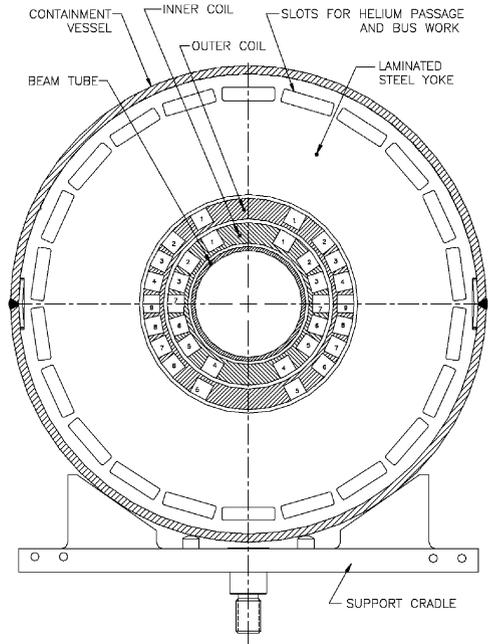
Fig. 55. Cross-section of the helical dipole magnet. The yoke OD is 356 mm. The innermost conductor is at an ID of 100 mm.
