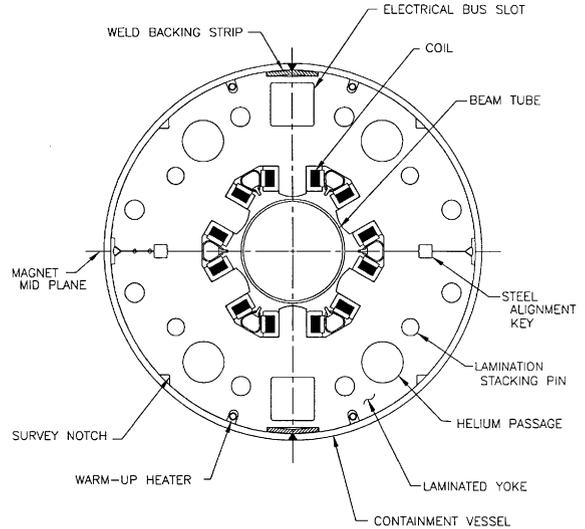
Fig. 19. Cross-section of the sextupole magnet. The coils are held in place by beryllium copper retainer springs and aluminum locking wedges (not labeled).
