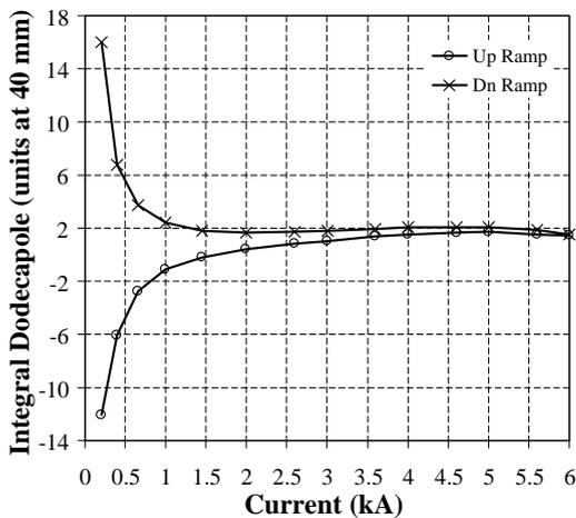
Fig. 37. Integral first allowed harmonic ( $b_5$ ) in Q3 magnet QRJ116.
