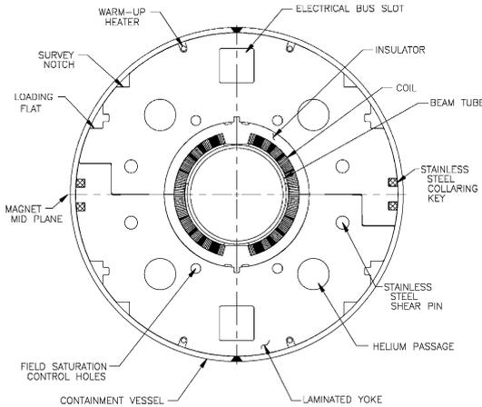
Fig. 41. Cross-section of the 100 mm D0 dipole magnet.
