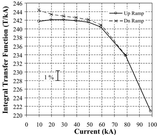
Fig. 23. Integral transfer function in trim quadrupole QRT148.
