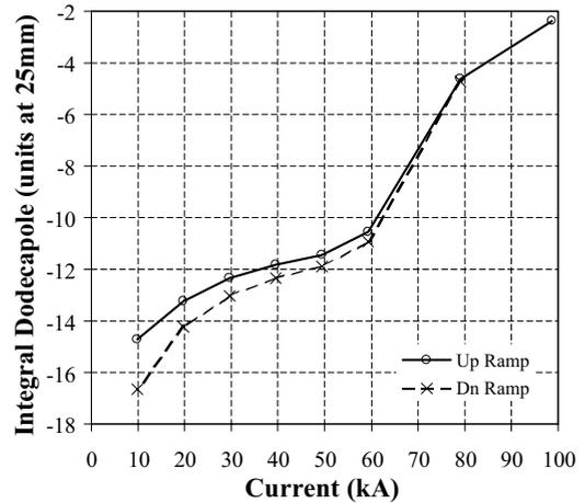
Fig. 24. Integral of the first allowed harmonic ( $b_5$ ) in trim quadrupole QRT148.
