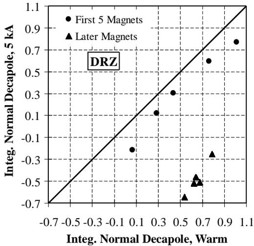
Fig. 47. Warm–cold correlation of the normal decapole harmonic ( $b_4$ ) in D0 dipoles.
