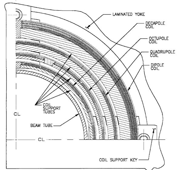
Fig. 26. A section of the 80 mm corrector magnet showing the coil layout in greater detail.
