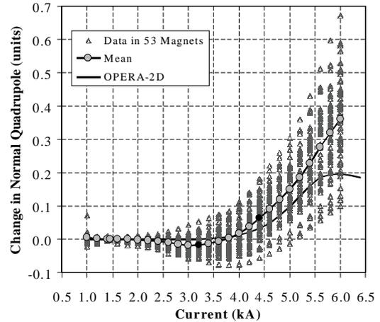
Fig. 8. Current dependence of the normal quadrupole component in the 80 mm dipole.
