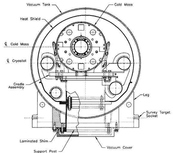
Fig. 2. A cross-section of the cryostatted dipole magnet. This section is at the magnet axial center, where the cold mass horizontal offset due to curvature is evident.
