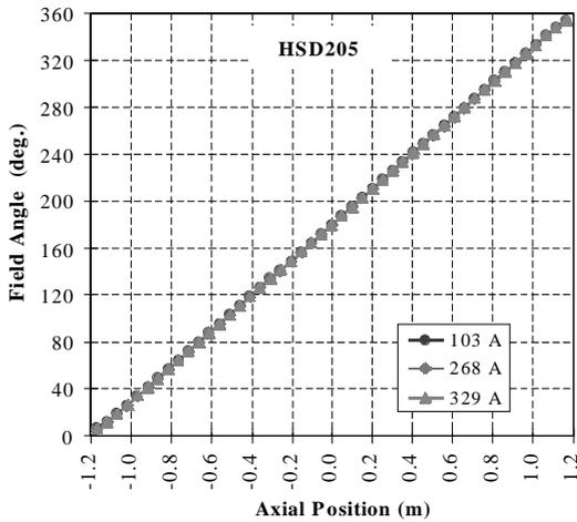
Fig. 63. Field angle as a function of the axial position in HSD205.
