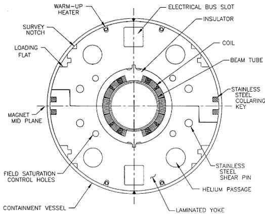
Fig. 1. Cross-section of the arc dipole magnet.
