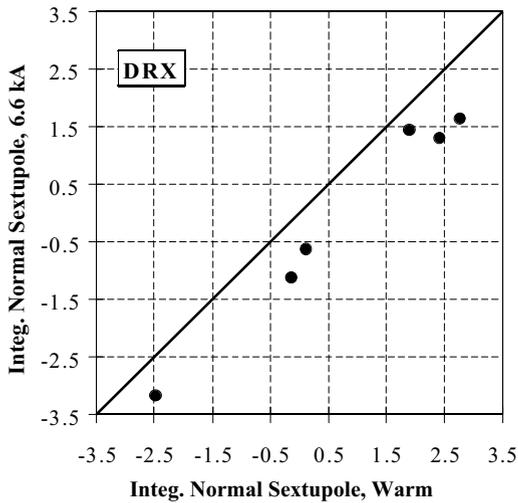
Fig. 54. Warm–cold correlation of  $b_2$  in DRX magnets.
