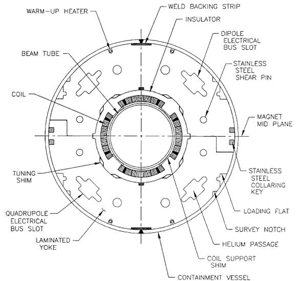
Fig. 30. Cross-section of the 130 mm quadrupole magnet.
