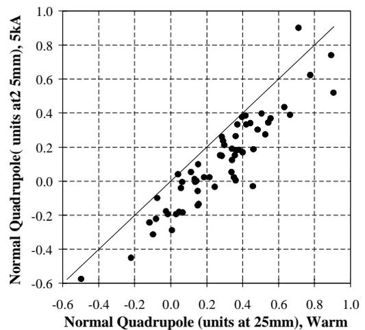
Fig. 4. Measured warm–cold normal quadrupole correlation.
