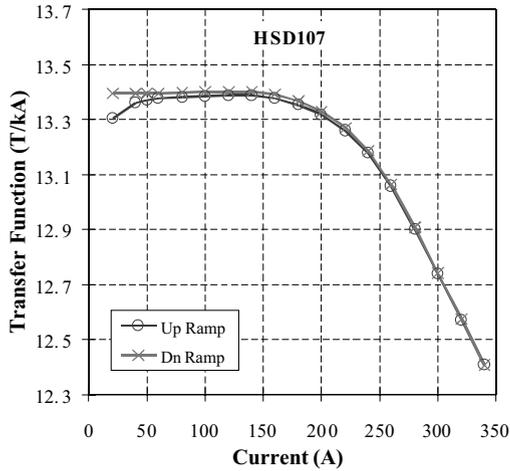
Fig. 59. Transfer function at the center of HSD107.
