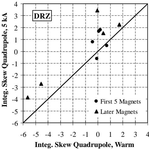
Fig. 44. Warm–cold correlation of the skew quadrupole harmonic ( $a_1$ ) in D0 dipoles.
