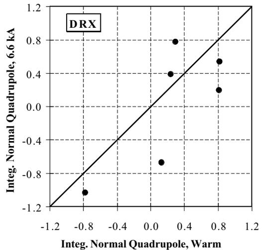
Fig. 53. Warm-cold correlation of  $b_1$  in DRX magnets.
