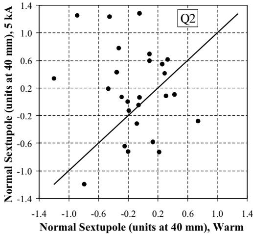
Fig. 40. Warm–cold correlation of  $b_2$  in the Q2 (QRK) magnets at 5 kA (shim saturation).
