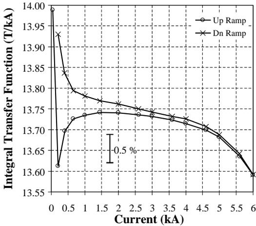
Fig. 32. Integral transfer function in Q1 magnet QR1114 (close to mean at 5 kA).
