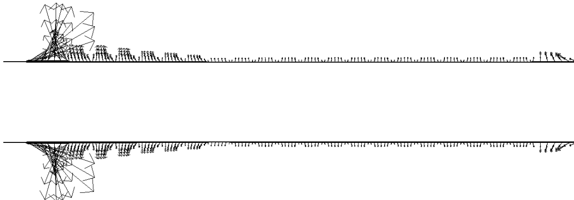
Figure 14.2 – Lorentz Forces from axisymmetric model, fields computed without iron.
