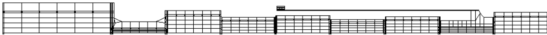
Figure 12.38 – Axisymmetric Model - 9 coils of the production solenoid are modeled. An additional 14 coils in the transport solenoid are included in the field and force calculation. These are “turned off” for the second load case. Plots of the models based on the use of internal mandrels are included with the discussion of the early results that used internal mandrels.
