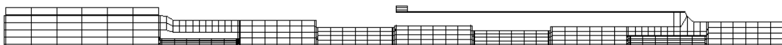
Figure 12.42 – Second Generation of Internal Mandrel Model, with reinforcements added to P1 and the thin coils , p2 and p8, Used in Run # prod02.
