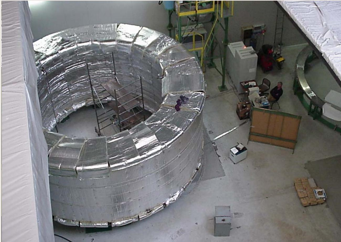
After impregnation the inner surface presented excess of resin needing to be removed
