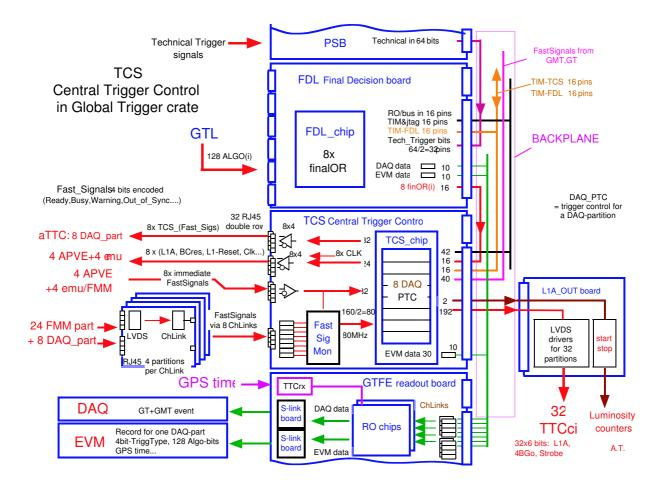
Fig. 3: Block diagram of TCS in Global Trigger Crate
