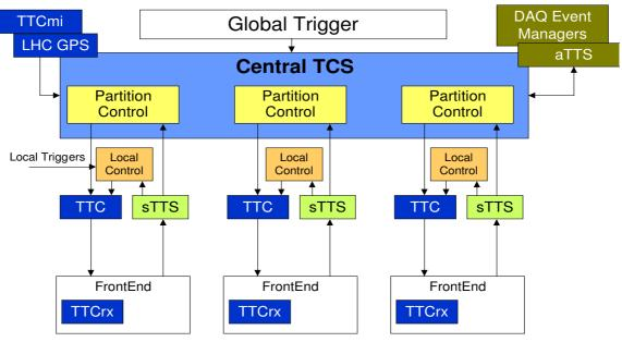
Fig. 1: Overview of the Trigger Control System.
