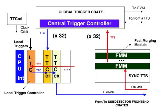
Fig. 2: Trigger Control Architecture.
