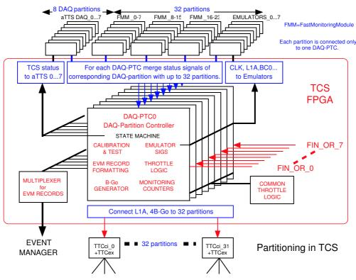
Fig. 4: Partitioning of the Trigger Control System.
