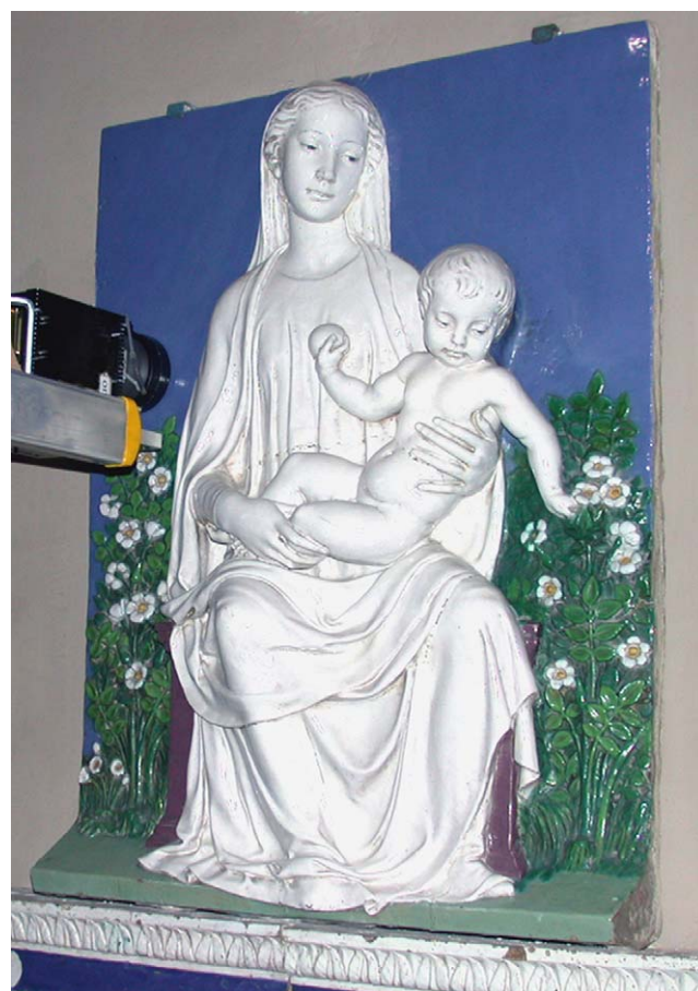
Fig. 4. The PIXE-alpha set-up during the analysis of the blue background of the Madonna del Roseto (Inv. n. 31), a 1460–70 Luca Della Robbia sculpture conserved in the Museo Nazionale del Bargello in Florence. The publication of the picture has been authorized by the Italian Ministero dei Beni e le Attività Culturali. Duplications or reproductions of the picture are forbidden.
