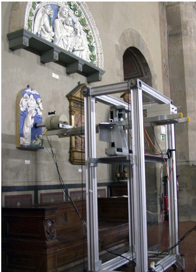
Fig. 5. A view of the equipment during the XRF analysis of the blue background of the Madonna che adora il Bambino (Inv. n. 21), a Luca Della Robbia sculpture conserved in the Museo Nazionale del Bargello in Florence. The publication of the picture has been authorized by the Italian Ministero dei Beni e le Attività Culturali. Duplications or reproductions of the picture are forbidden.
