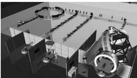
Figure 8. The Heidelberg Ion-Beam Therapy Centre features two horizontal beams and a carbon ion gantry, the first one ever built (HIT Photo Gallery).
