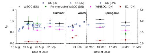
**Figure 4.** The f<sub>M</sub> determinations of different carbon fractions with combined measurement uncertainties for daytime (D), nighttime (N), and whole-day (DN) samples. Horizontal bars mark beginning and end of aerosol collection.
