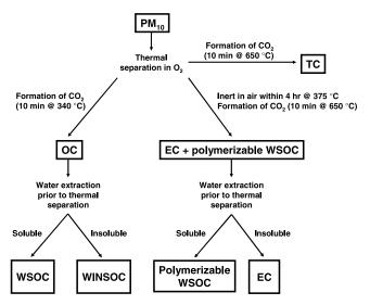
**Figure 1.** Separation scheme of the different carbon fractions. The <sup>14</sup>C was directly measured in OC, WINSOC, EC, and the mixture "EC + polymerizable WSOC." The <sup>14</sup>C values in WSOC and polymerizable WSOC were deduced from subtraction. Modified from *Szidat et al.* [2004c].
